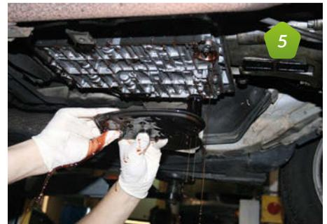
**3** Although most ATF will be in the gearbox itself, the torque converter also holds a significant amount – usually around 1½ - 2 litres – and this should therefore also be drained if at all possible. The problem, though, is that Mercedes-Benz don’t always provide a drain point, and the provision or otherwise isn’t 100% age or model specific! To find out if yours has one prise out these rectangular plugs...
