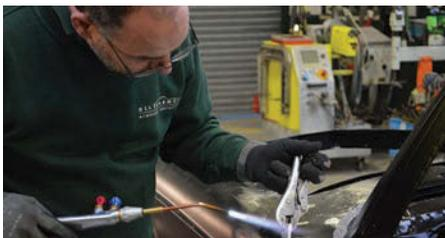
*Using often forgotten, traditional techniques such as lead loading allows us to complete our restorations to the most original and exacting standards possible.*
