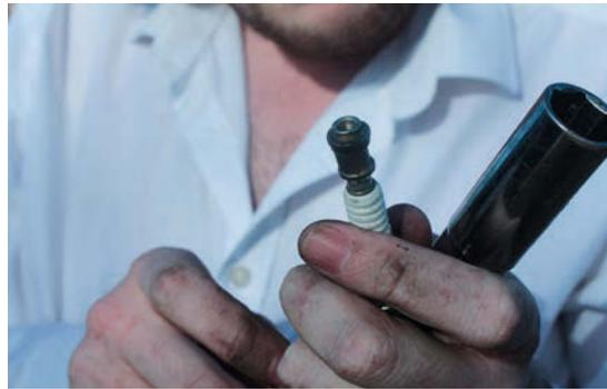
**Left:** Bits of lead had melted onto the plugs
