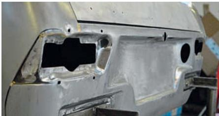
*Using often forgotten, traditional techniques such as brazing allows us to complete our restorations to the most original and exacting standards possible.*
