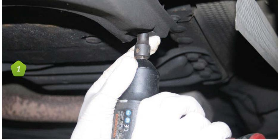
**1** First job – obviously – is to remove the engine undertray – held on by 8mm bolts in our case. There are usually two trays – one under the gearbox and one under the engine – and while you can access the gearbox with just the rear tray dropped, you’ll need to turn the engine in a minute, and this is generally easier from underneath and with both undertrays off.
