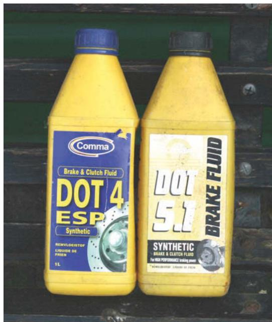
**Above:** DOT4 and DOT5.1 brake fluid – the latter has a higher boiling point and was originally specified mainly for sports/performance cars. This particular bottle of DOT 5.1 is, though, way past its use-by date.
